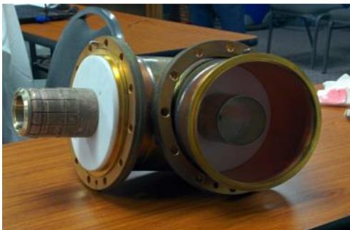
6 1/8 inch hardline connector (72 ohms)
